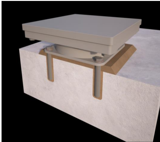
Large stanchion baseplates
