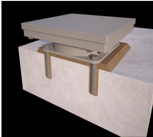
Stanchion baseplates where a large gap is present
